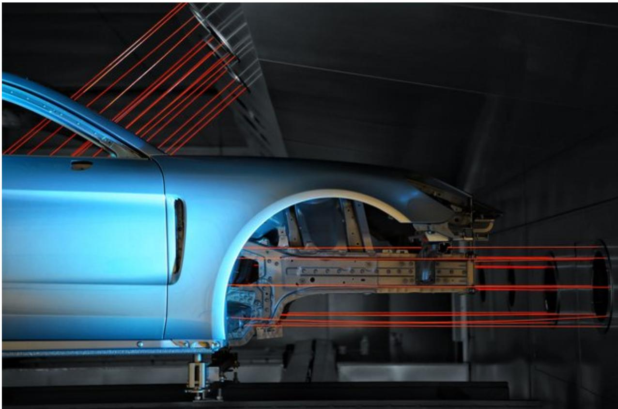
With EcoInCure, hot air flows in through the windshield. This leads to the car body panels being heated from the inside out.
